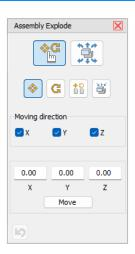
Select a part by clicking on the model. Move the cursor onto a part of the model in the display and move the part while pressing the left mouse button. In this mode only single parts can be moved.
