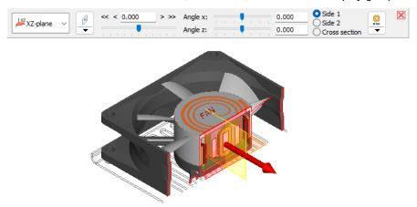
After activating the tool, the model will be displayed sectioned. The section settings are shown in the top of the display. The cross section controls are shown in the display in front of the model.
