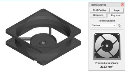
This function calculates the surface area of all models that is projected onto one of the three standard planes. This, for example, is needed to calculate locking forces when making molds.
