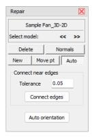
Click the Auto tab to automatically repair inverted faces and open edges.
